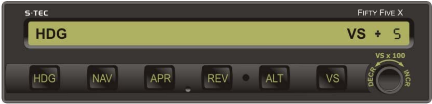
Fig. 3-12. AP Display, HDG and VS Modes Engaged
