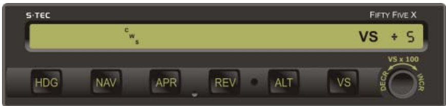
Fig. 2-9. AP Display, CWS Mode Engaged, 500 FPM Climbing (Pre-Flight)
