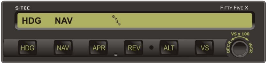
Fig. 3-10. AP Display, HDG Mode Engaged, NAV GPSS Mode Armed
