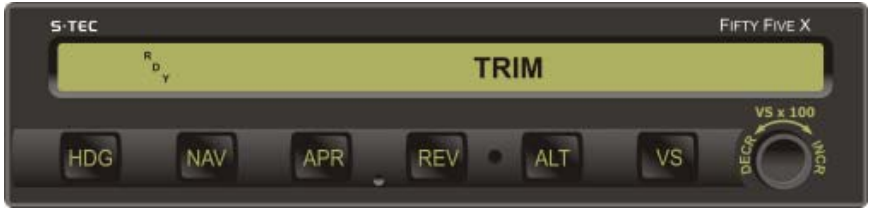
Fig. 2-15. AP Display, Manual Electric Trim in Progress (Pre-Flight)
