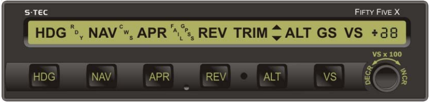
Fig. 2-1. AP Display, All Annunciations at Power-Up
