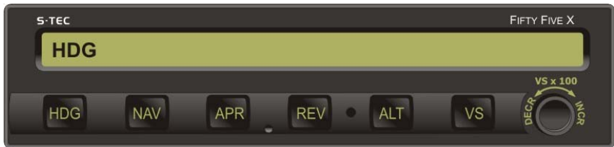
Fig. 3-1. AP Display, HDG Mode Engaged
