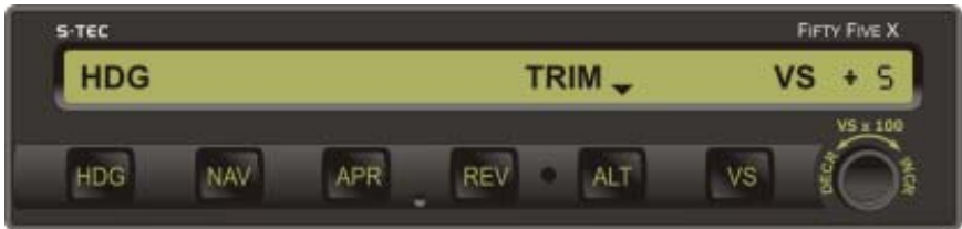
b. TRIM DN in Progress
