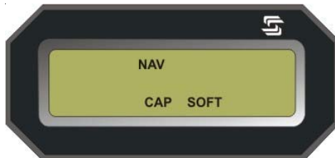
Fig. 3-4. Remote Annunciator Display, NAV Mode Engaged, CAP SOFT Condition
