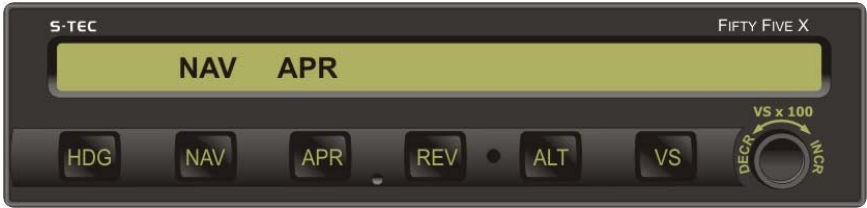
Fig. 3-6. AP Display, NAV APR Mode Engaged
