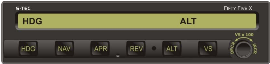
Fig. 3-11. AP Display, HDG and ALT HOLD Modes Engaged
