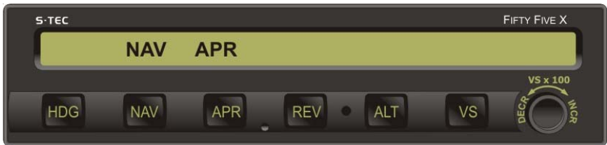
Fig. 3-27. AP Display, NAV APR Mode Engaged, Track LOC Front Course Inbound
