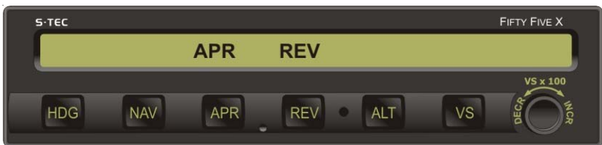
Fig. 3-21. AP Display, REV APR Mode Engaged, Track LOC Back Course Inbound
