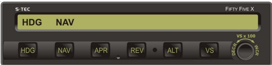
Fig. 3-8. AP Display, HDG Mode Engaged, NAV Mode Armed
