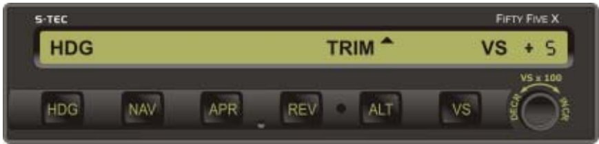
a. TRIM UP in Progress
