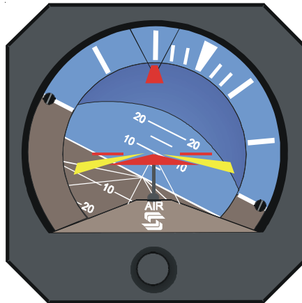
Fig. 3-39. FD Display, FD/AP Mode Engaged
