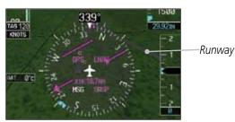
Figure 5-44 Depiction of Runway Not in Loaded Flight plan
