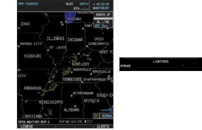
Figure 4-100 GFDS Data Link Lightning and Legend
