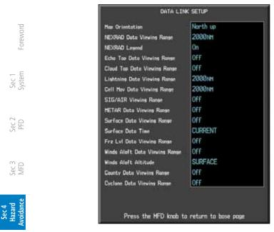
Figure 4-21 Weather Data Link Setup Menu Options
