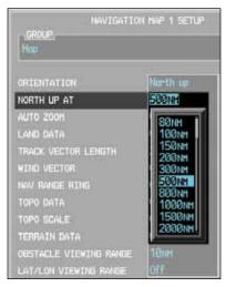
Figure 3-18 Navigation Map "North Up At" Orientation Range Selection
