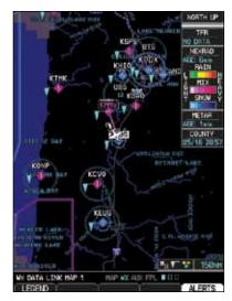
Figure 4-39 XM Weather - Graphic METARs
