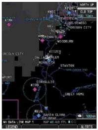
Figure 4-31 XM Weather - Cloud Tops
