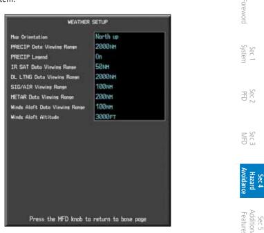
Figure 4-85 Weather Data Link Setup Menu Options
