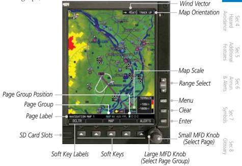
The nose of the aircraft icon is placed on the Navigation Map at the location or responding to the calculated present position. The start of corresponding to the calculated present position. The aircraft position and the flight plan legs are based on information received from the currently selected GPS navigator. The leg of the active flight plan currently being flown is shown as a magenta line on the navigation map. The other legs are shown in white.
