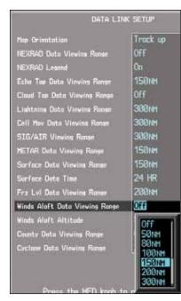
Figure 4-52 Winds Aloft Data Viewing Range Selection
