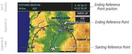
Figure 3-12 Bearing/Distance Measurement
