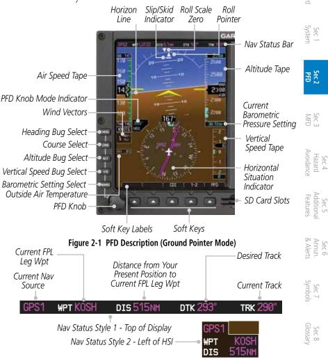
**NOTE:** When navigating to a waypoint very far away, the DTK, CRS, and TRK values displayed on the GDU 620 may differ from the on the navigator, however the CDI is correct and is the primary means of navigation. This is because the GDU 620 applies magnetic variation corrections for the current aircraft location, but some navigators apply magnetic variation correction for the waypoint location.
