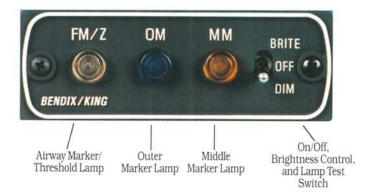
The self-contained KR 22 Marker Beacon unit is a crystal controlled superheterodyne receiver which provides accurate visual and aural indication of passage over 75 MHz beacons located on airways and ILS approach courses.
